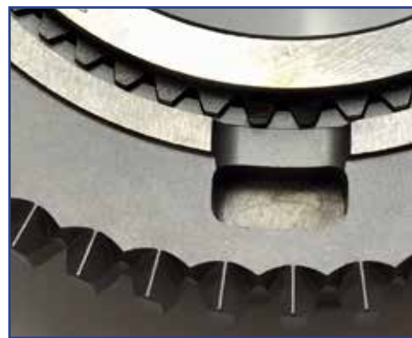
HOLINGER 3rd gear uses positive, splined connection to prevent failures
